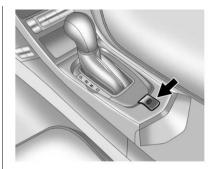
Vehicles with the electric parking brake (EPB) have a switch in the center console.
